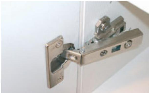
**GB** To mount the doors, clamp the hinge into the mounting plate on the carcass.
